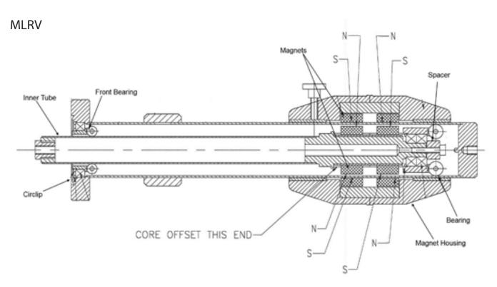
Please note only the bearing sets and outer tube are interchangeable between the MLRM (Obsolete) and the MLRV.
